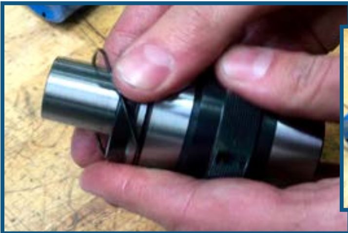
STEP 6: Remove O-Ring from Chuck and move Jaws to the forward position.
