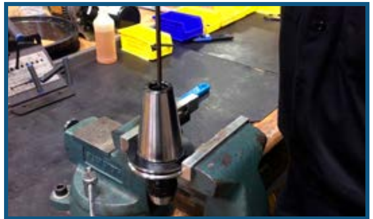
STEP 2: Loosen the Draw Screw halfway.
