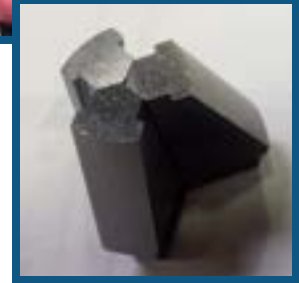
STEP 10: Once cooled, remove old Jaws and replace with new Jaws.
