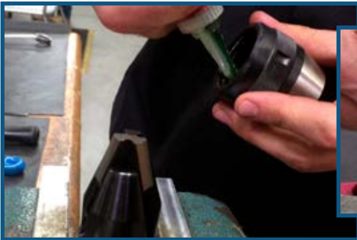
STEP 11: Apply Loctite (Semi-Perm) to threads and tighten down the Nose Cone.
