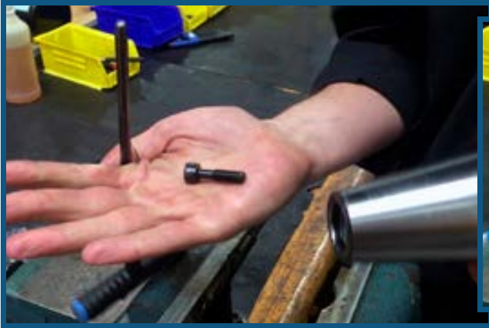
STEP 5: Remove the Pull Stud, Spacer, Draw Bolt and Chuck from the Taper portion.
