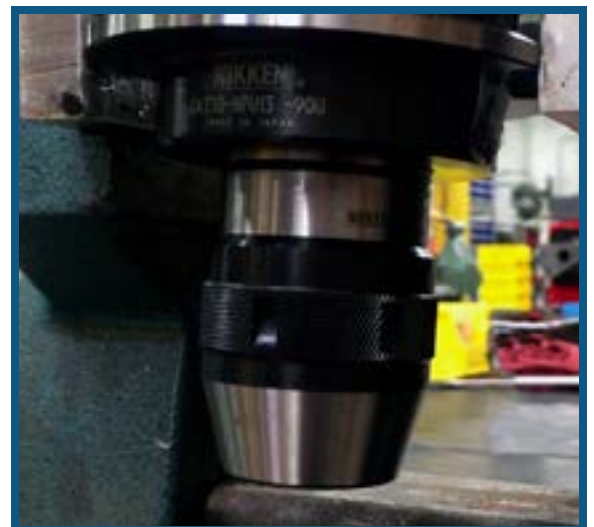
STEP 4: Tighten Pull Stud until Chuck is pressed on Taper.
