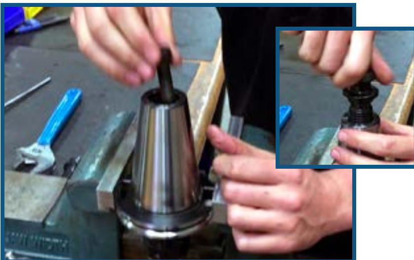
STEP 3: Insert Spacer and replace the Solid Pull Stud.
