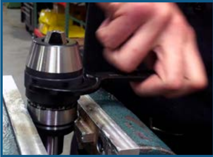
STEP 9: Use Spanner Wrench to remove the Nose Cone and expose the Jaws.
