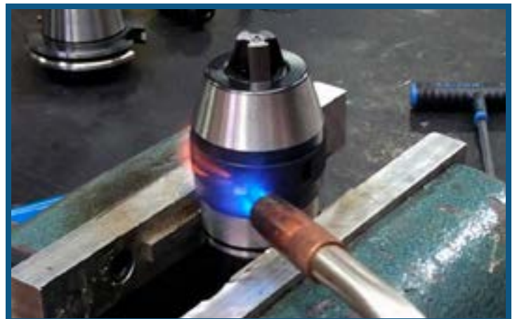
STEP 8: Heat the Nose Cone to burn off Loctite.
